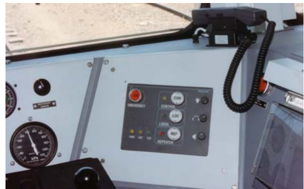
Figure 4 CountryNet Driver's Console – satellite and terrestrial systems are integrated, with a simple interface
