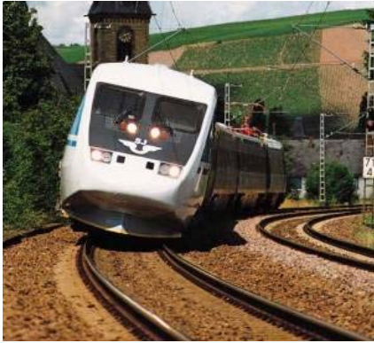
Figure 9: Tilting Train - showing the difference between a "comfort" speed and a "derailment" speed
